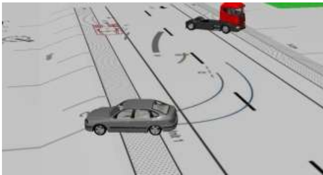
Figure 12. An example of a 3D Simulation in PC-Crash using the scene diagram shown in Figure 5 .
