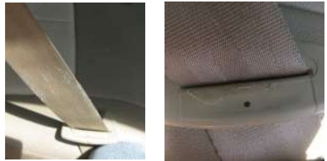
Figure 10. Seat belt webbing found stretched (left), and melting of the seat belt buckle seen due to usage by the occupant (right).
