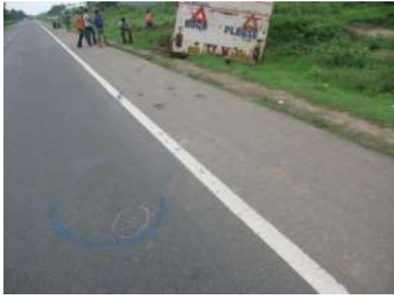
Figure 19. Pictures showing the final rest position of the vehicles (top) and a gouge mark indicating the point of impact (bottom).
