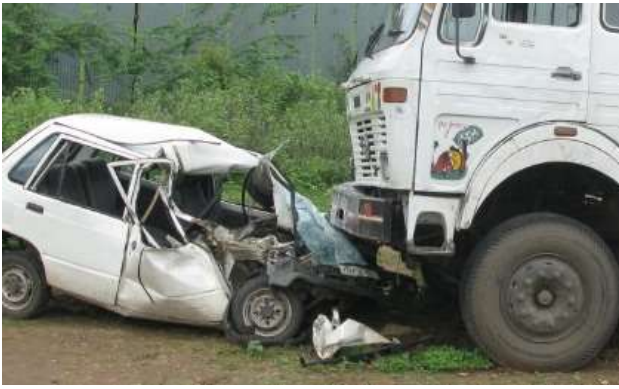
Figure 20. Intrusions of the car caused due to underride with the truck.
