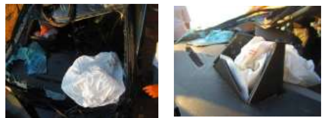
Figure 11. Deployment of airbags (left); Tear points being inspected (right).
