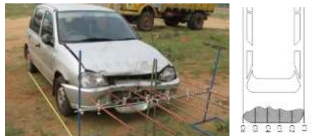
Figure 8. Crush profile being measured on a passenger car using crush jig.
