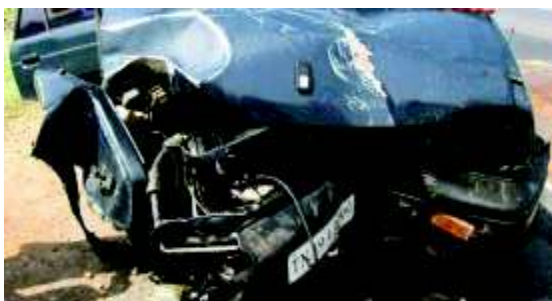
Damage to a car after collision with a concrete pole
