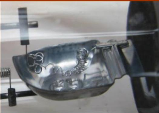
however, when it is at an incandescent temperature, the filament would be smooth and susceptible to shape changes. So when there is a shock at the time of crash, the filament would be likely to uncoil (*left*), showing deformation at one or several points.
